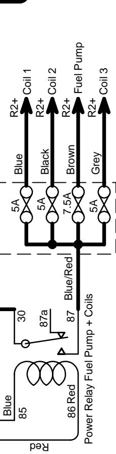
Connect supply wires at the battery terminal !!
